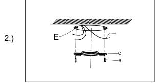
Step 2. Mount the mounting bracket (C) to the junction box(E), using mounting screws(B).
